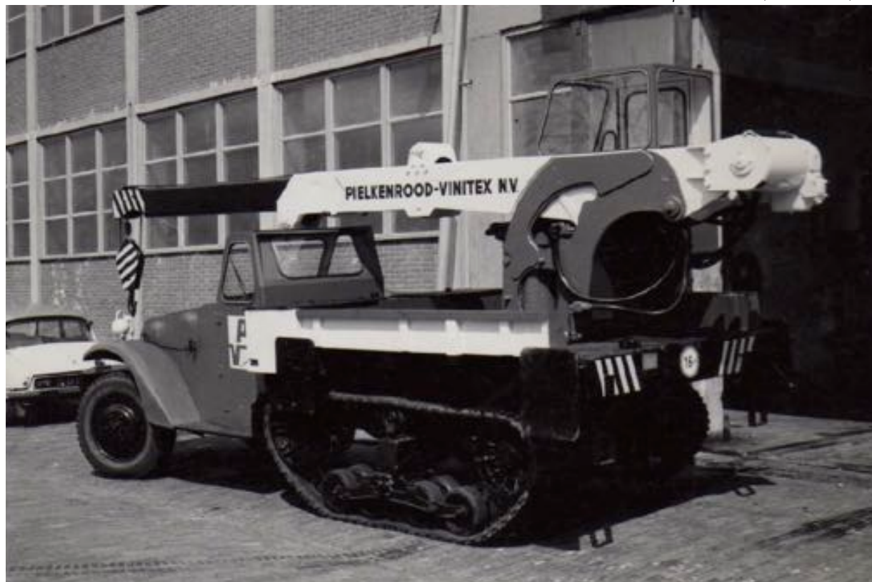
Austin-Western kraan op half-track (Foto KENZ)
